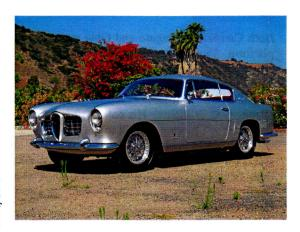
The 1900 was the first series of Alfa Romeos built on a standardized production line and they were also Alfa's first production car without a separate chassis as well as the first Alfas offered with left-hand drive steering configuration.
